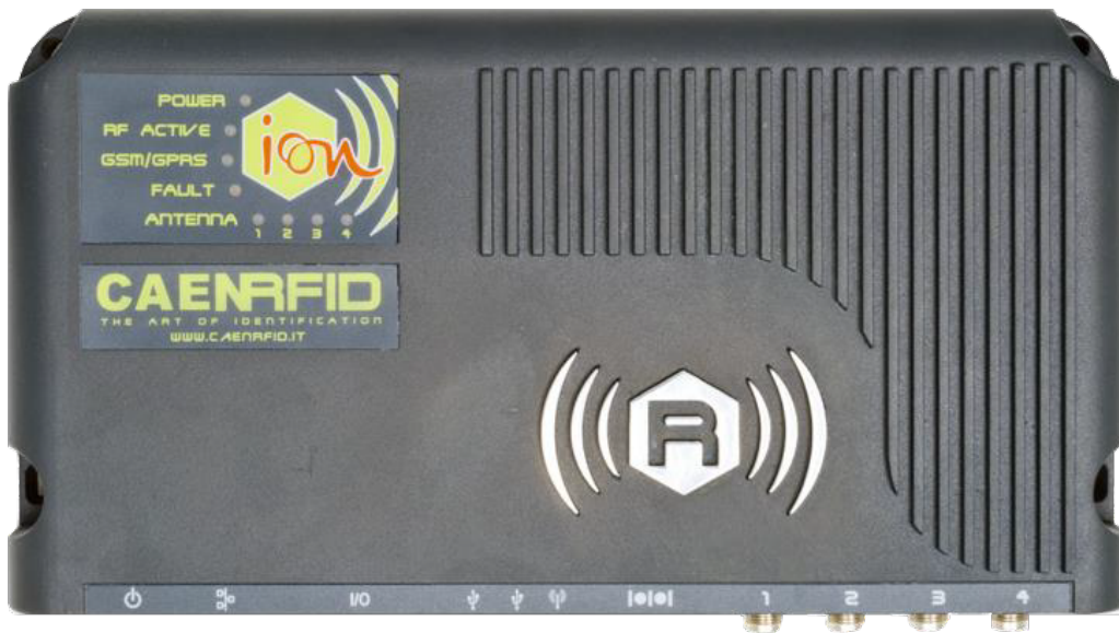
Fig. 3.9: Ion R4301P Top Cover LEDs
