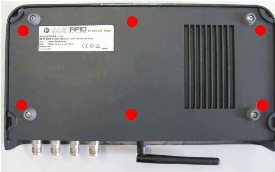
Fig. 10.1: Bottom cover screws position
